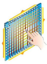
Embedded IR sensors inside the touch frame emit and receive invisible infrared light beams in front of the computer imaged surface. Whenever your finger or an object breaks through this light grid, it is seen as a touch point which is same as a left mouse click. Your touch can also perform all the standard tablet gestures and multi touch functions
