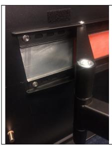
Once inserted, line up left edge of heater plate with left edge of interior mount
