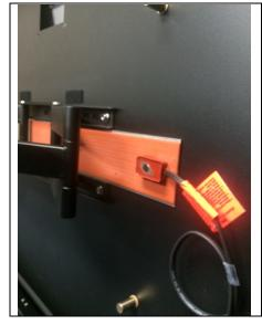
Insert Heater behind interior mount as shown
